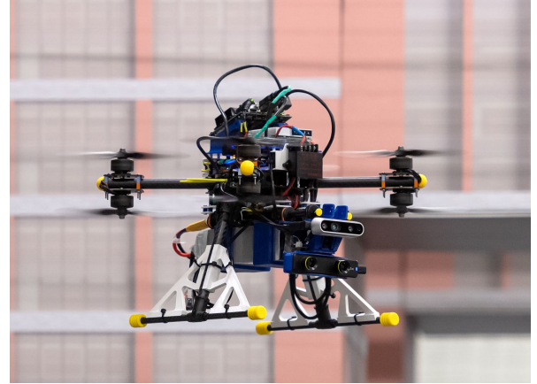
Fig. 4. Autonomous coaxial octocopter, integrating an Nvidia Jetson Orin NX, a Stereolabs ZED Mini, and an Intel RealSense D435i depth camera, explores and navigates through an unknown environment.
